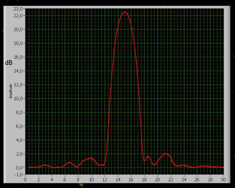
Measurement of low level broadband noise is better with large bandwidth
